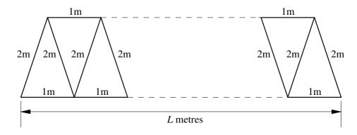
The diagram shows wooden beams which support the roof of a house.
